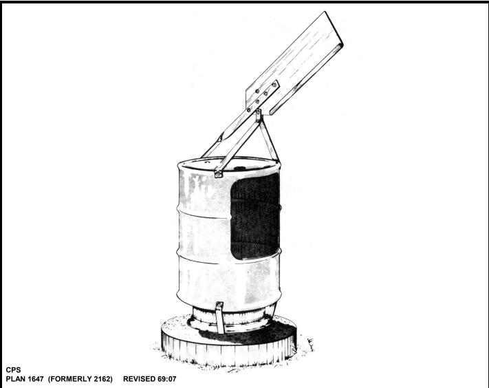
Details for a rotating mineral feeder are given on the back of this leaflet. This useful item of feed lot or pasture equipment is assembled from common hardware items including a standard steel drum and used automobile parts. Wind rotates the drum so that
