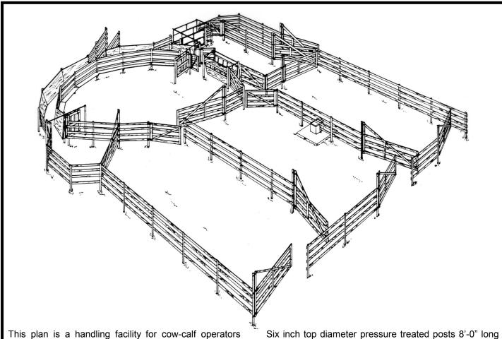
This plan is a handling facility for cow-calf operators and feedlot operations. A loading chute, squeeze, headgate, and scale is incorporated in this facility. The scale and scale cage is offset from the main working chute.
