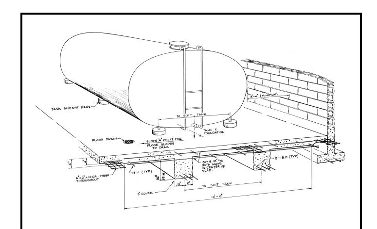
This leaflet shows foundation details for bulk milk tanks up to 11,500 litres. The leaflet shows round tank support pads to facilitate easy cleaning.
