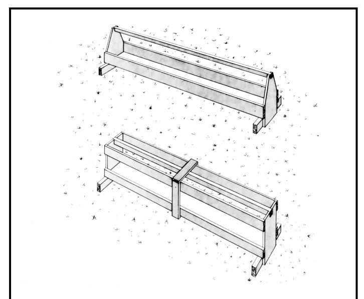
The back of this leaflet gives details for building two simple grain feed troughs suitable for lambs. These feeders may be located in field, feedlot or finishing pen. Each foot of double-sided feeder length will serve two lambs (group feeding all at once) or 6 lambs if self-fed continuously.
