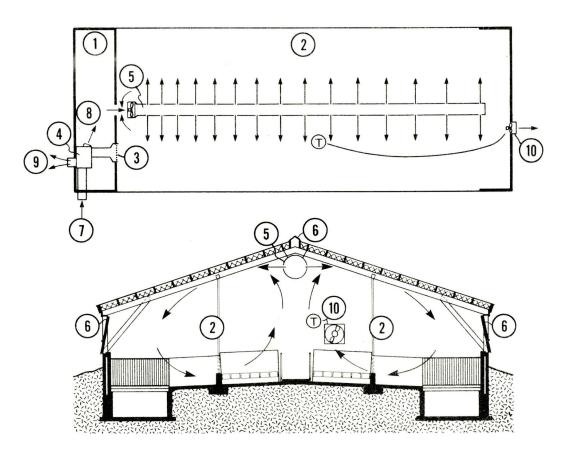
The smooth, high cathedral ceiling of this plan is uniquely adaptable to a combined natural/mechanical ventilation system. The ability to add required supplemental heating at one convenient point in the air supply system is a distinct advantage of the powered winter ventilation. The extra mechanical parts of this system may cost little more than full automation with compressed air (or other automatic systems) for controlling the sidewall and ridge vents.
