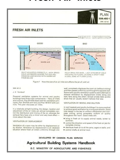
Powered ventilation systems for animal and poultry buildings have three main components - fans, air inlets and controls. Plan 9700 deals with fan ventilation principles and Plan 9705 deals with fans. This plan discusses air inlets. In a relatively airtight building, the design, location and adjustment of air inlets can almost completely control the distribution and mixing of the air, whereas the exhaust fans have only a minor and very local effect.
