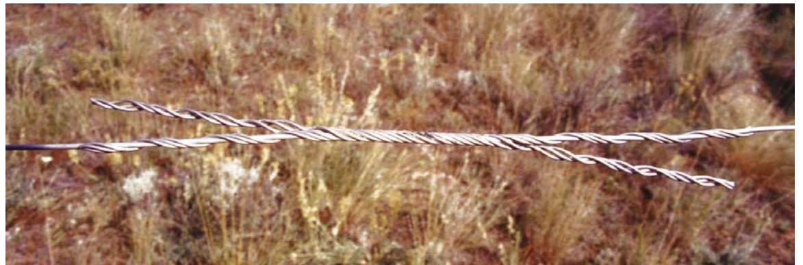
Figure 6 Mechanical Splices for High Tensile Smooth Wire
