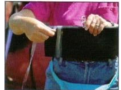
wrapping chip tape for ease in handling; cut at board edge
