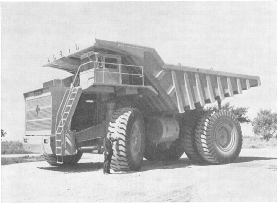
Plate VIII A. Lectra Haul dump truck of 200 tons capacity used by Kaiser Coal Ltd. at its Harmer Ridge strip mine. This is currently the world's largest two-axle truck.
