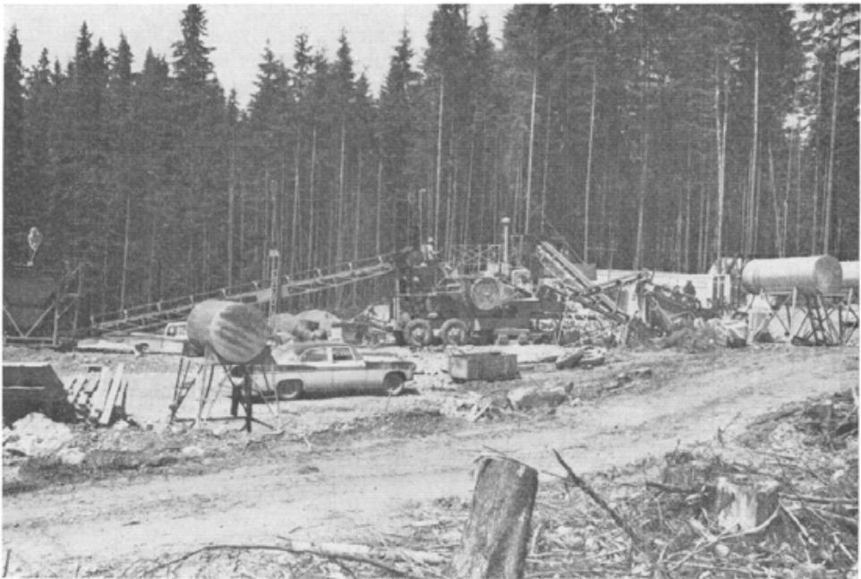
Plate IIb. Crushing and splitting bulk samples at sampling plant at Island Copper.
