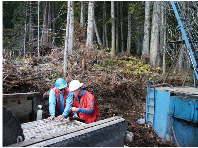
Photo 7. Diamond drill core from the copper-gold Northeast zone at the Mount Polley mine.
