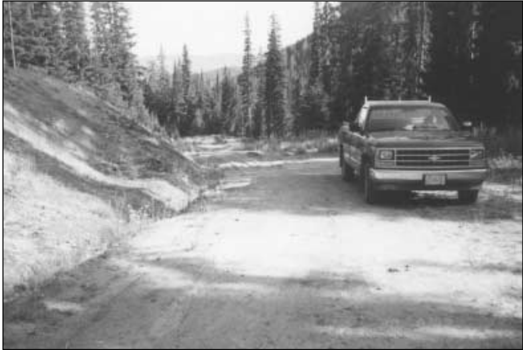
Figure A3.4. Example of sediment production class 4 (sediment production = 70 m 3 /km/yr).
