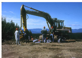
Hoe with various head attachments, VH mulcher on the ground in front of the hoe
