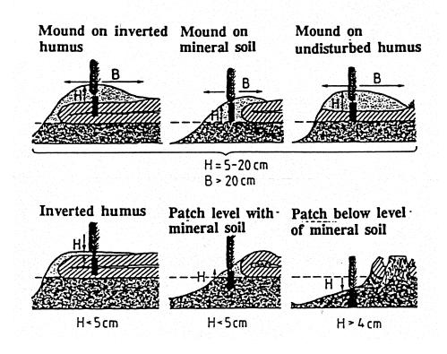
Figure 2: Sketches of the principles of the defined planting spots. H gives average height and B width in the figures. The dotted line shows the mineral soil level A negative value of H indicates that the spot is below this level.
