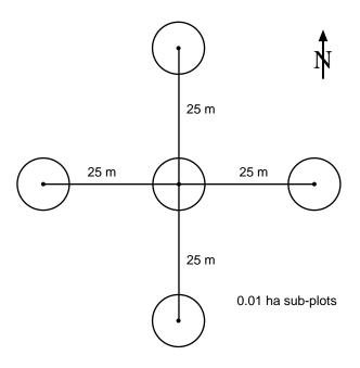
Figure 2. The layout of sub-plots in the cluster sample.
