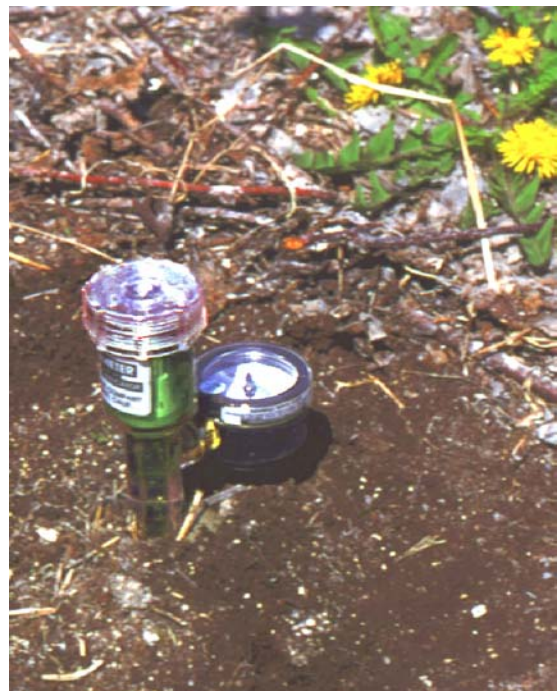
Figure 1 Tensiometer in the soil after installation
