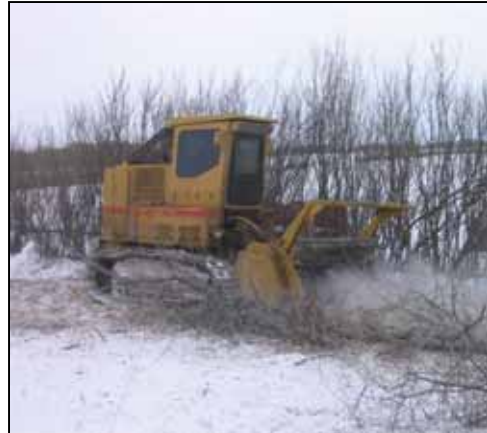
Picture of a mid-size mulcher (400hp).
