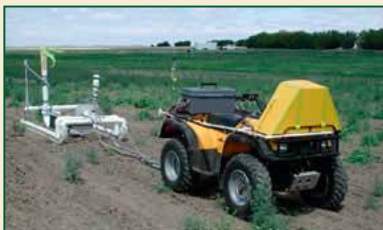
Sledded dual EM38 salinity meters with standard base station setup
