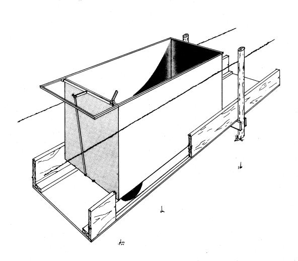
This leaflet plan provides details for constructing a metal, bottom unloading, feed cart and wood feed bunk. The feed cart and feed bunk are sized to provide a matched unit.
