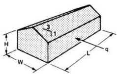
For rectangular farm storage buildings with stud walls and gable truss roofs as above, the maximum hourly wind pressure is:
