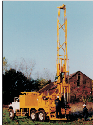
Figure 4. Example of Truck-mounted Drill Rig
