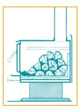
Burn Short, Hot Fires: Build a small, hot fire first to preheat the firebox and chimney. Open the damper wide to help fuel the fire; leave open for about 30 minutes. To gain the most heat from each load of firewood, the wood should be flaming throughout the burn cycle until it is reduced to charcoal. You should periodically inspect your stove or fireplace to ensure a continued safe and clean-burning operation.
