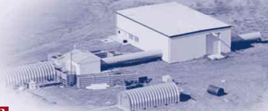
Below: This blast tube is used in evaluating protective equipment and investigating blast effects on the human body, using dummies. Explosive force of up to 100 pounds-per-square-inch can be simulated in the tube.
