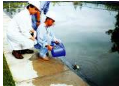
Periodic collection of sample to ensure the effluent is within the internationally acceptable standards
