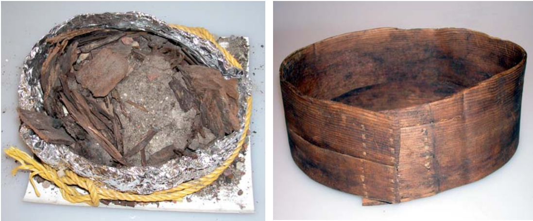
Untreated wooden object 18 th century irreversibly damaged Treated bowl 18th century using PEG and freeze-drying
