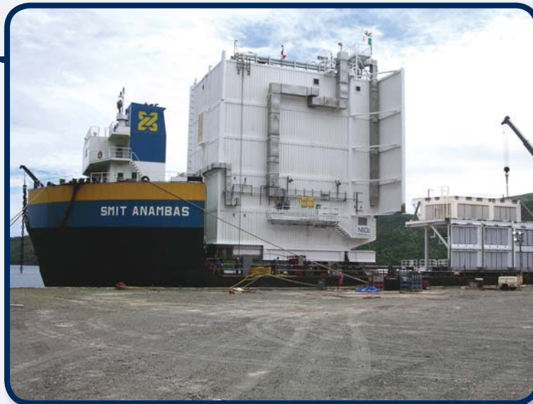
Additional Living Quarters and the Starboard Lifeboat Enclosure loaded onto a barge in Bull Arm
