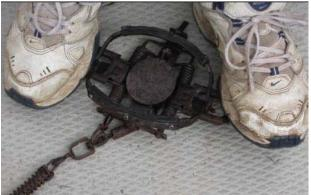
Your weight on the levers will relax the pressure on the trap jaws, loosening the jaws and enabling your dog to pull its foot free.
