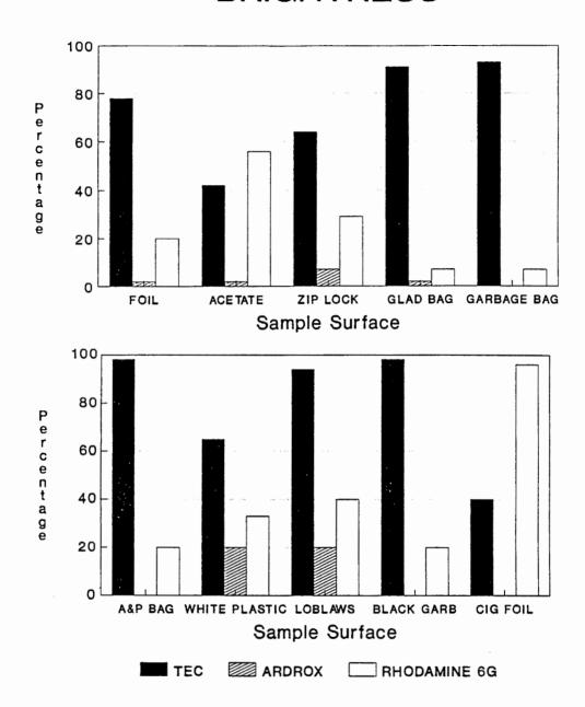
Figure 5 Percentage scores for print brightness for all ten surfaces. TEC (solid), Ardrox (hatched) and Rhodamine 6G (blank).
