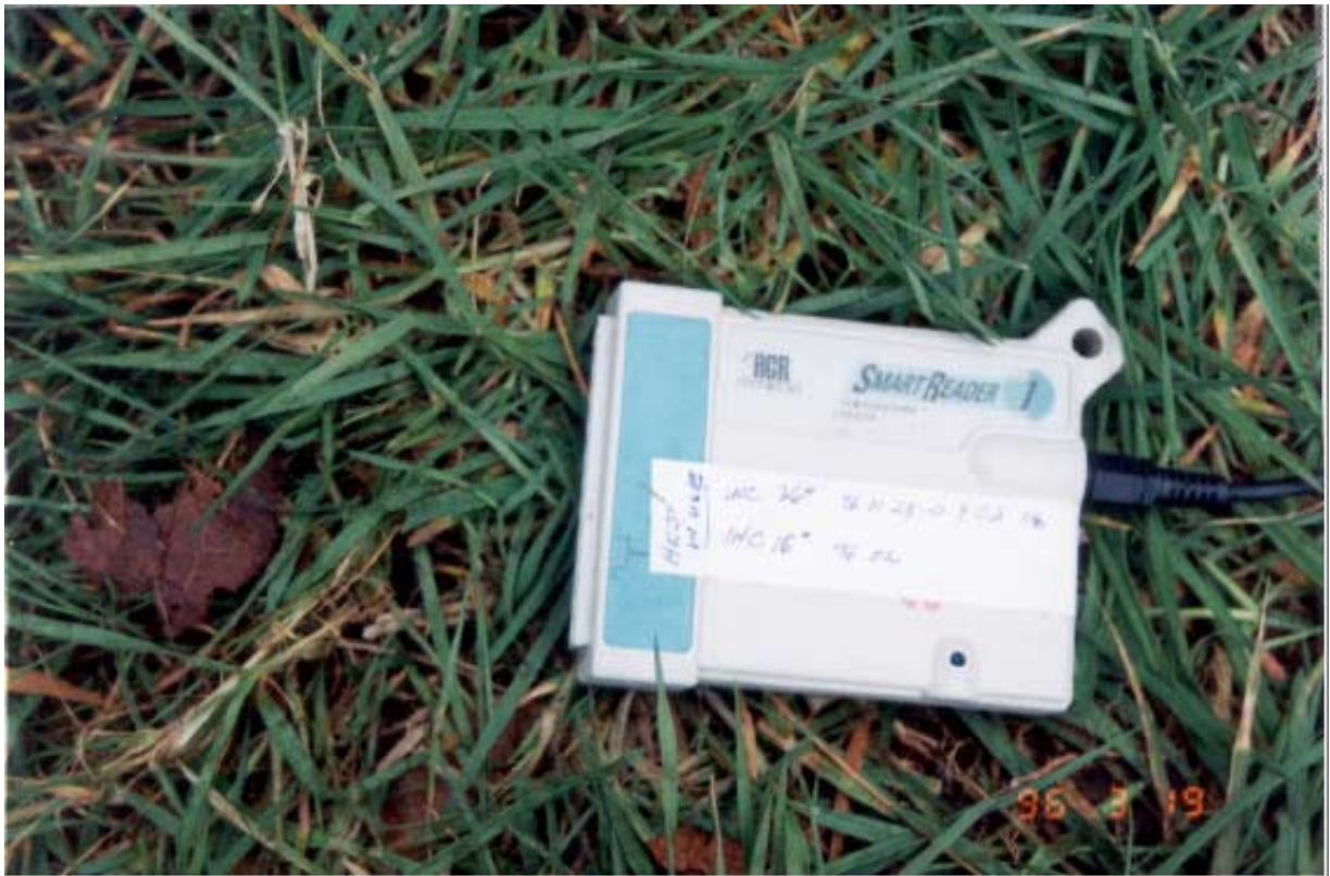
Figure 22 Smart Reader Datalogger
