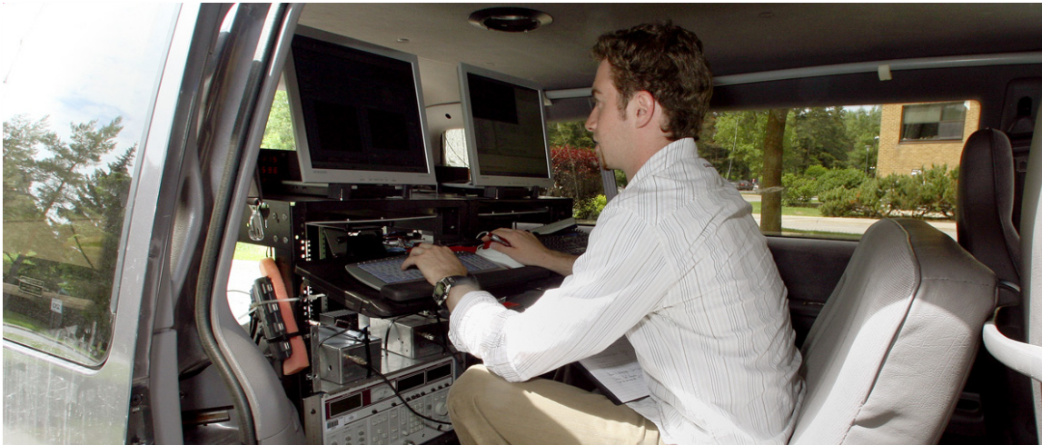
Phillippe Gandy works in a CRC test vehicle, equipped with a complex antenna system that allows the reception of DAB at vehicle speeds higher than what the current standard allows.
