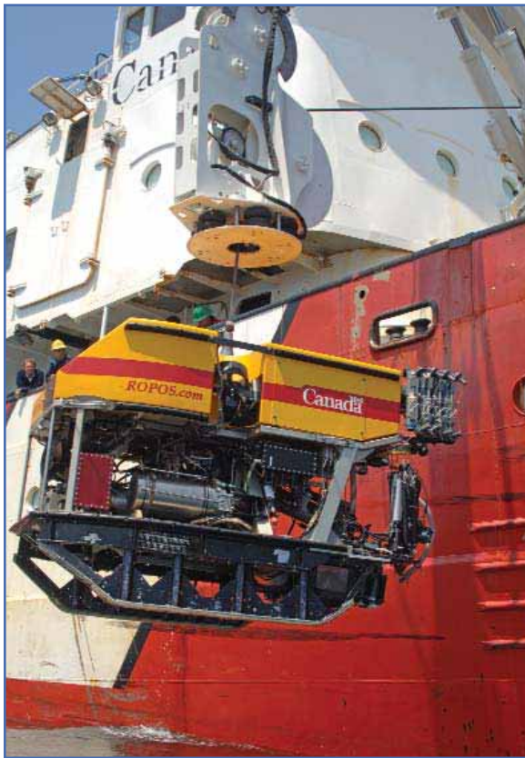
A Remotely-Operated Platform for Oceans Science (ROPOS) is used to explore the ocean floor as deep as 2,500 meters beneath the surface
