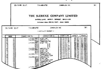
**Memory Reception.** Guarantees information will never be lost if the FAX-L6500 runs out of paper. Up to 32 transactions (up to 800 pages) can be stored in memory, which print out automatically when the paper is replaced.
