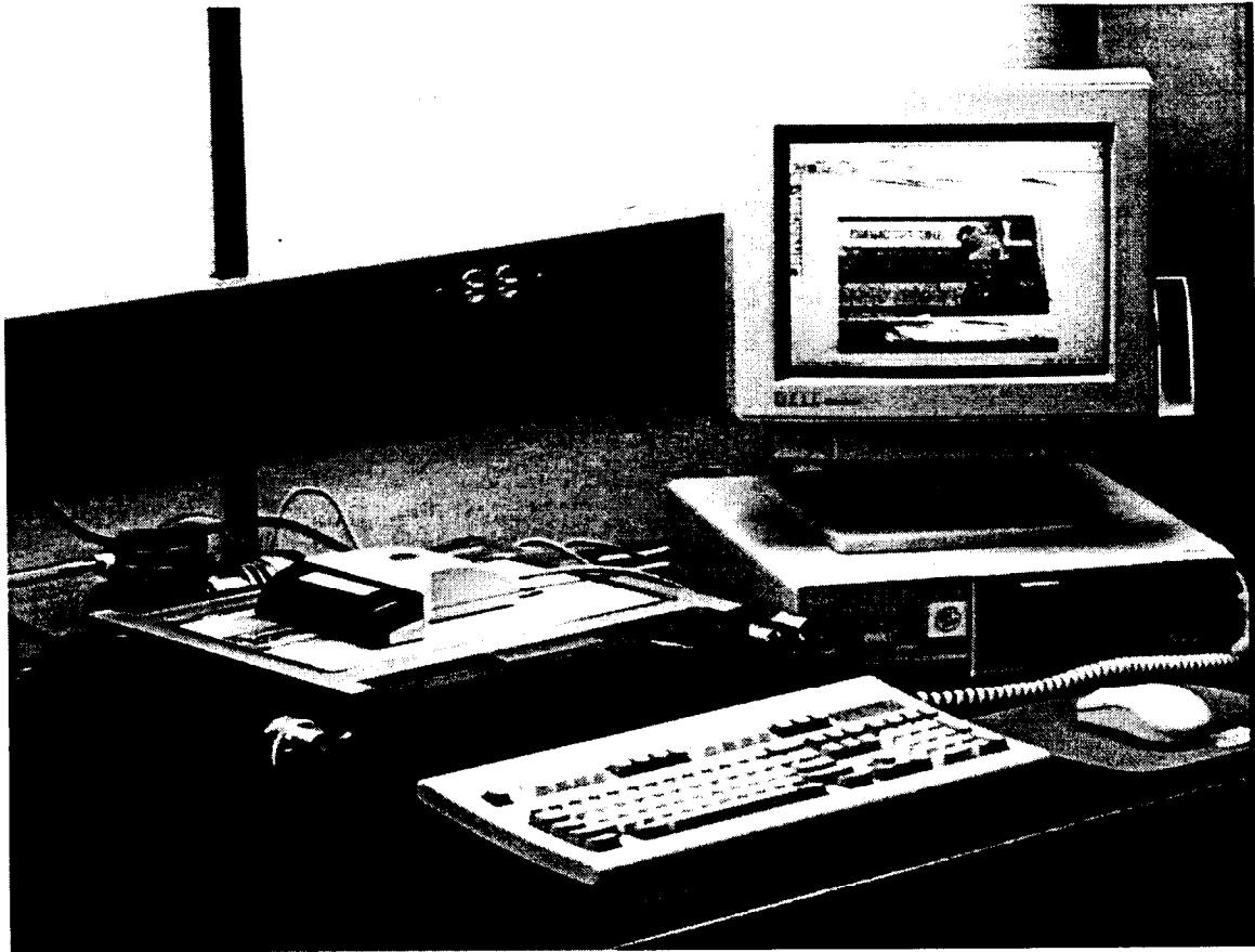
Figure 17. EOL handheld scanner on Solid Film Highlighter vacuum table with PC host computer.
