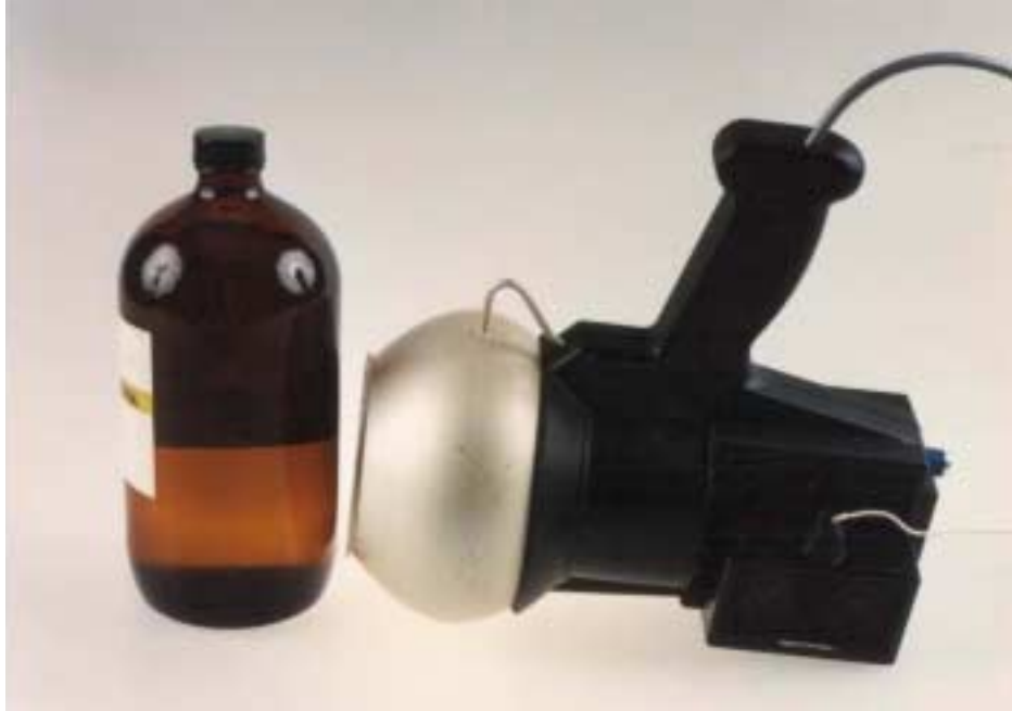
PHOTOGRAPH 1 - The M600P being used on a bottle containing a liquid
