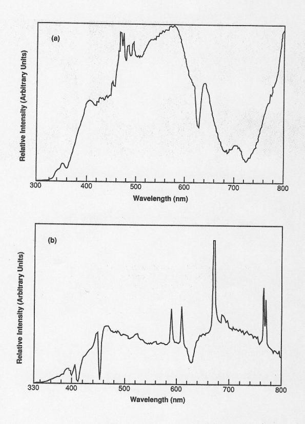
Figure 1 Corrected Spectral Output (a) Xenon Arc Lamp of the Polilight through the infrared filter (b) Indium MARC Lamp of the Luma-lite
