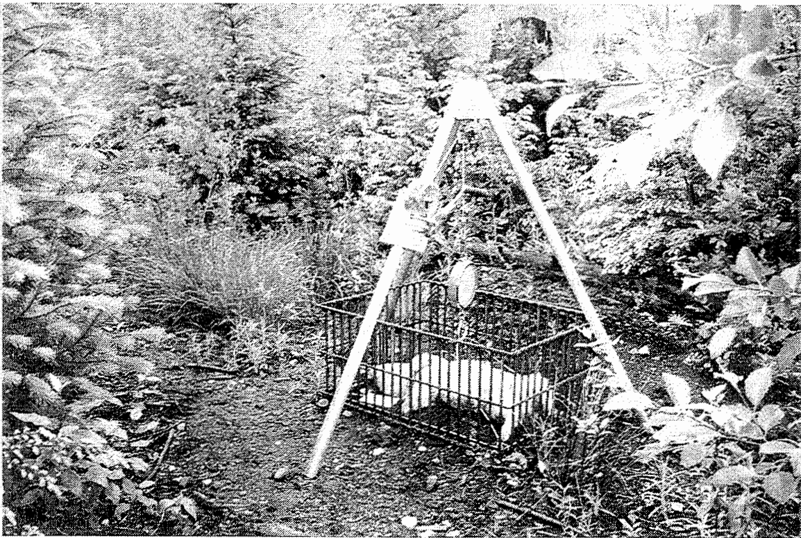
Figure 8 Photo: Weighing Platform
