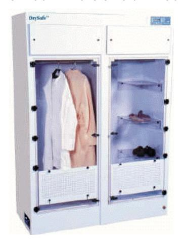
This cabinet protects evidence from airborne and cross-contamination while eliminating the odours and bacteria associated with process. The units are configured to clean the incoming "drying" air through HEPA filtration and filter the cabinet exhaust through combination of carbon and HEPA filtration. This combination assures evidence integrity without compromising the well being of co-workers.
