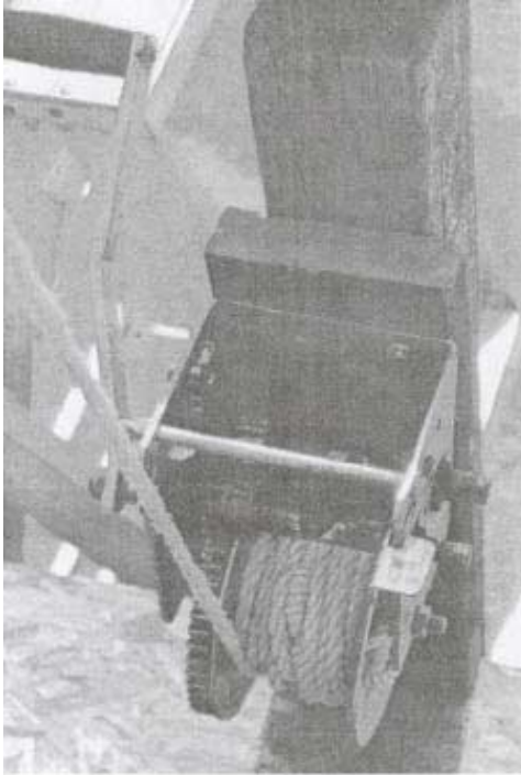
Photo 1. Winch connected to main rope.
