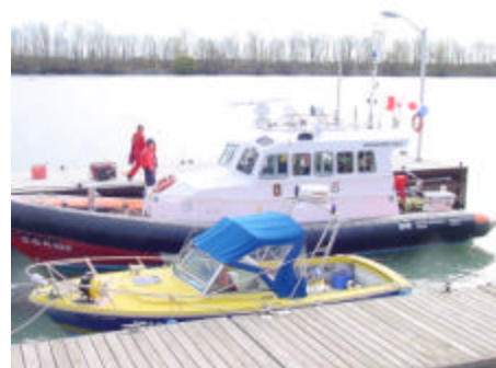
The NRPS 24' Limestone in the foreground was used to tow the Klien 595 Sonar Towfish. Note the small generator mounted on the bow to power the electronic equipment.
