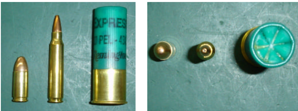
Figure 4.1: Bullet Types used for Ballistic Evaluation (9mm, 5.56mm & #4 Buck round)
