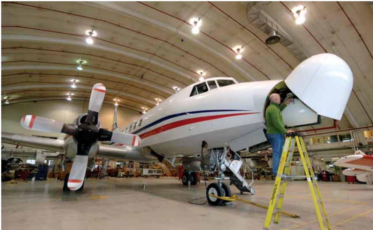
The XWEAR radar is installed on the Convair 580 during the SWATHBUCKLER experiment
