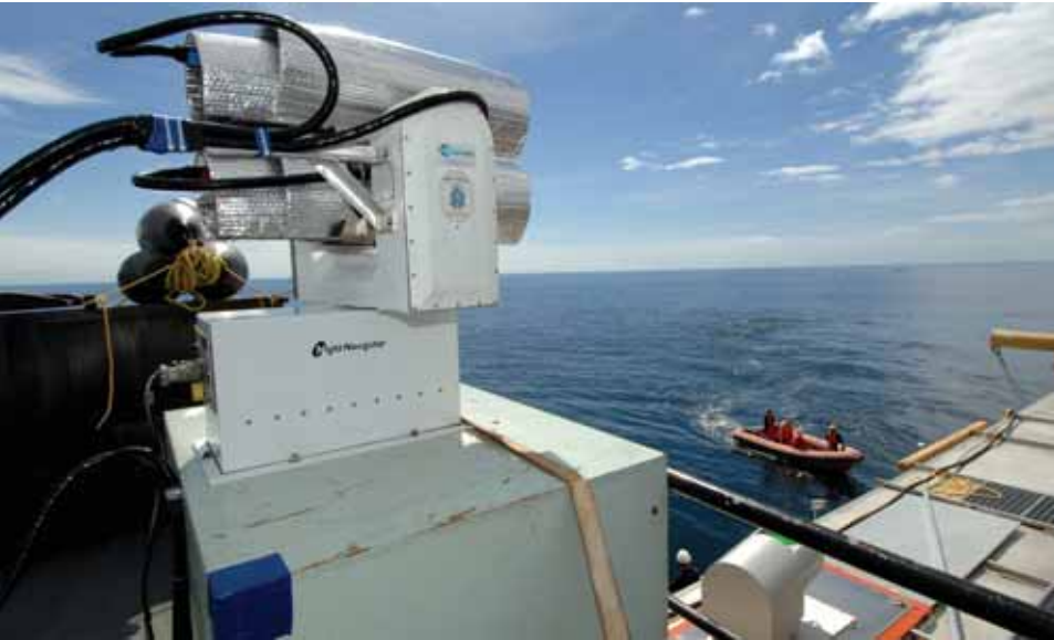
Infrared cameras on board the CFAV QUEST acquire images of small targets during the SISWS trial
