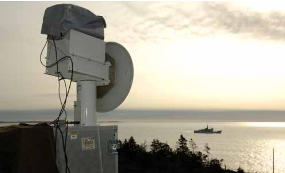
Measuring the radar cross section of CFAV QUEST during the SISWS trial
