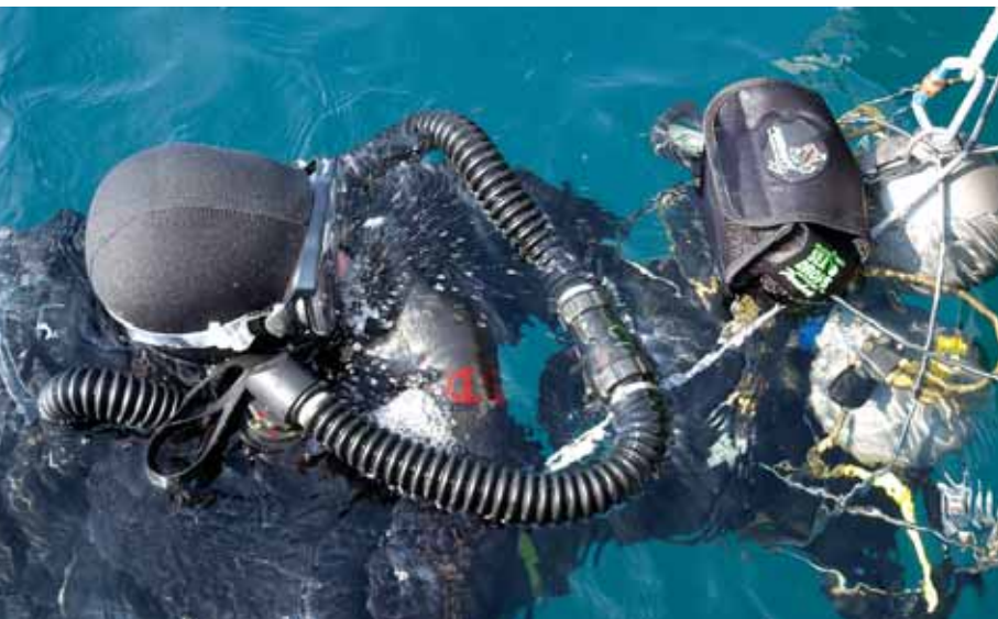
DRDC diver tests the Auxiliary Gas Supply
