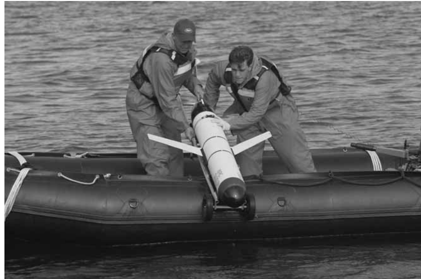
Deploying the SLOCUM glider during the MarSIE trials. Photo: Don Glencross, DRDC
