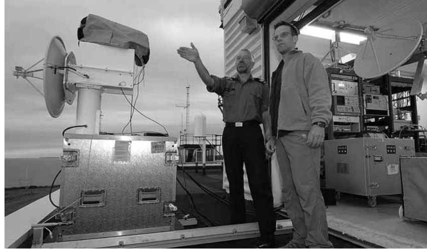
Working with the radar cross section measurement equipment during the SISWS trial. Photo: Janice Lang, DRDC
