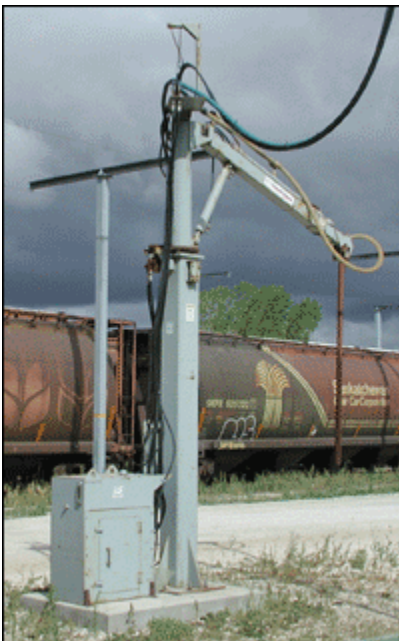
Figure 8.4: Pneumatic probe sampling unit
