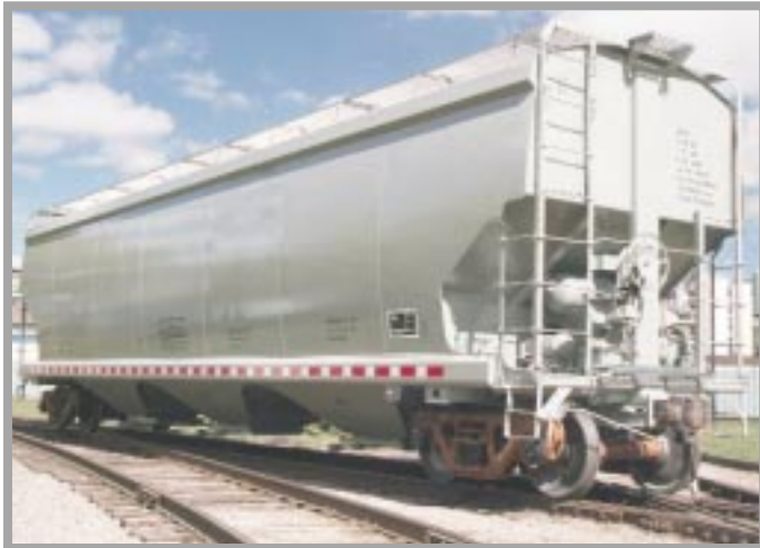
Covered hoppers provide maximum cubic capacity and increase shipping efficiency for such products as potash, grain and salt. (Photo: National Steel Car Ltd.)
