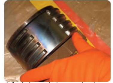
A fuel channel closure plug is inspected prior to labelling, transport and storage for later refurbishment.
