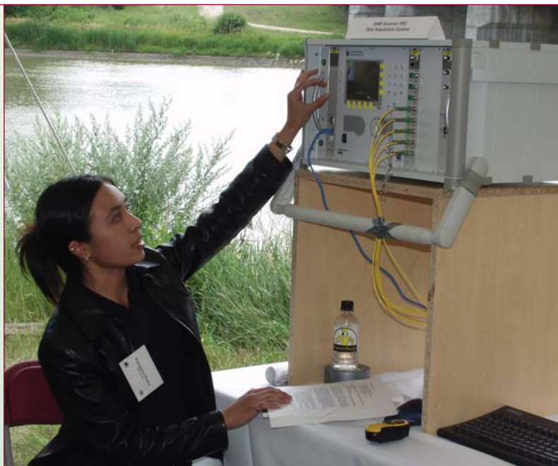
ISIS researcher Evangelina Rivera field tests the IDERS system at the Taylor Bridge in Headingley, Manitoba, on July 31, 2003. The high-tech box reads data from ISIS-developed “smart” sensors that measure stress levels in bridges and other structures.
