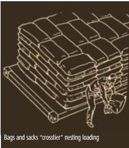
Fill side and end voids to prevent movement of cargo.
