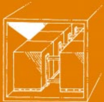
Fill side and end voids to prevent movement of cargo.
