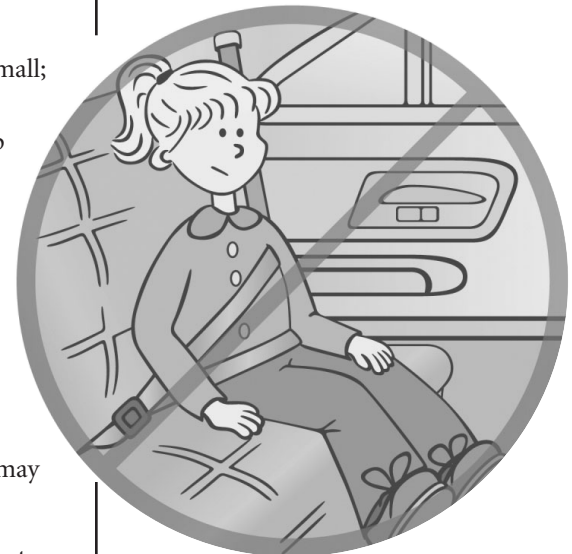
It is dangerous to put the shoulder belt behind the back or under the arm
