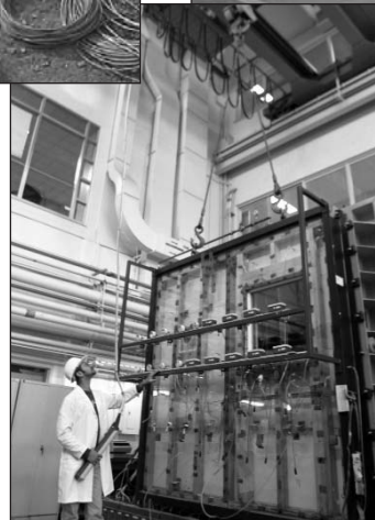
Wall and window assemblies being prepared for water entry experiments on the NRC-IRC Dynamic Wall Test Facility
