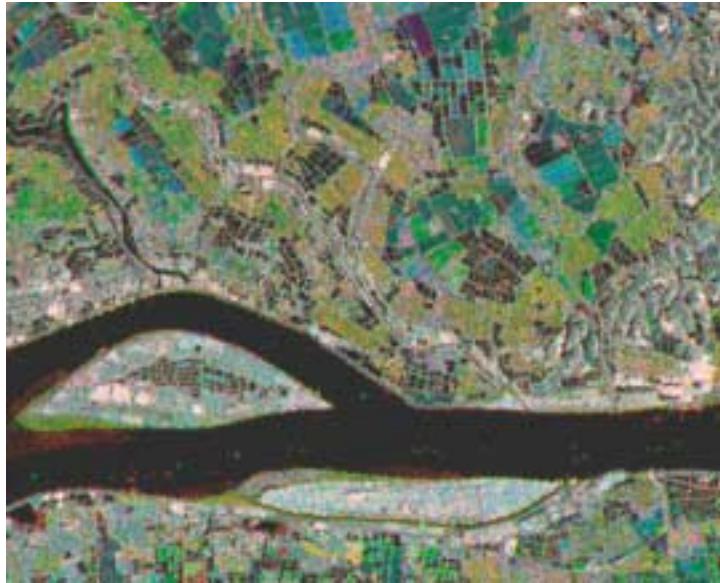
False colour composite using three RADARSAT images of the Zhao Qing area in the Guangdong Province of China. (© CSA 1996. Received by CCRS. Processed and distributed by RSI.)
