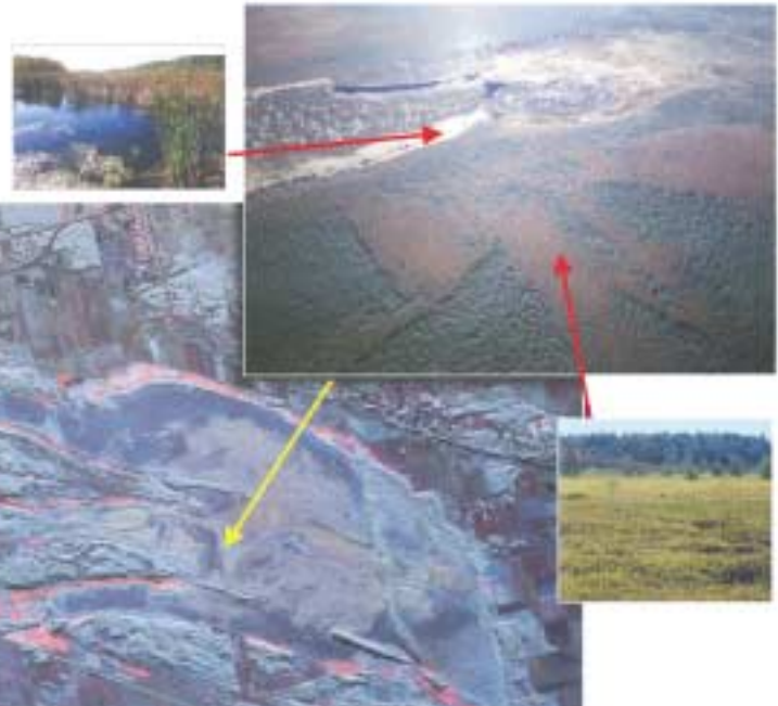
Wetland mapping using composite image of Mer Bleue using multi-polarization data. (© CCRS. Acquired by CV-580 C-band SAR. Processed and provided by CCRS.)
