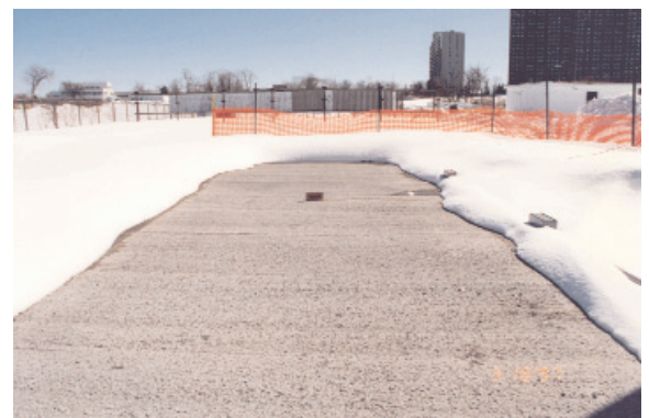
Test of a snow melting application
